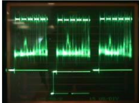
Fig. 4 PEC levels set correctly with headroom
