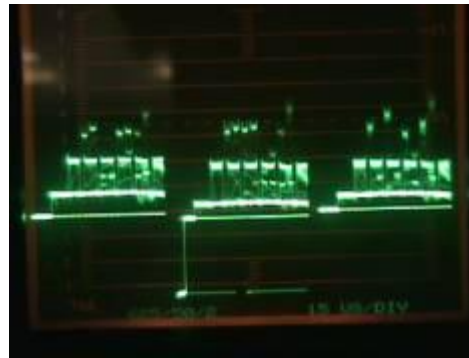
Fig. 14 PEC levels set correctly with headroom
